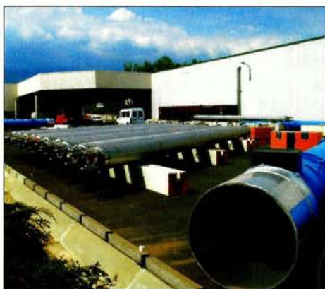
LHC dipole magnet cold masses awaiting installation into their cryostats at CERN.
