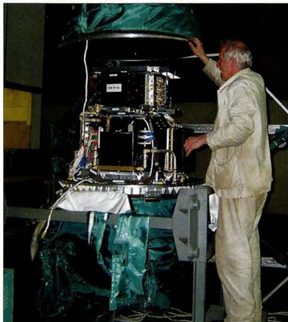
The mass and thermal model of the PAMELA experiment, inserted into the pressure vessel that will be attached to the Resurs-DK1 satellite, shows what this experiment to investigate antimatter in cosmic rays will look like when it is launched later this year. (PAMELA collaboration.)
